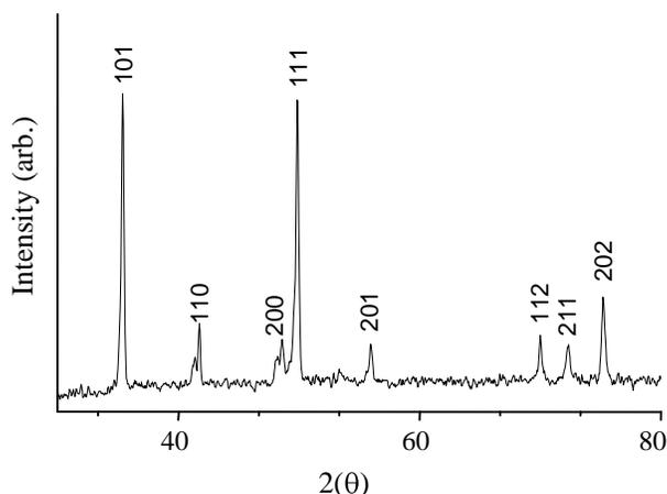
Figure 1. XRD pattern of as-cast  $\text{SmCo}_5$  alloy.
