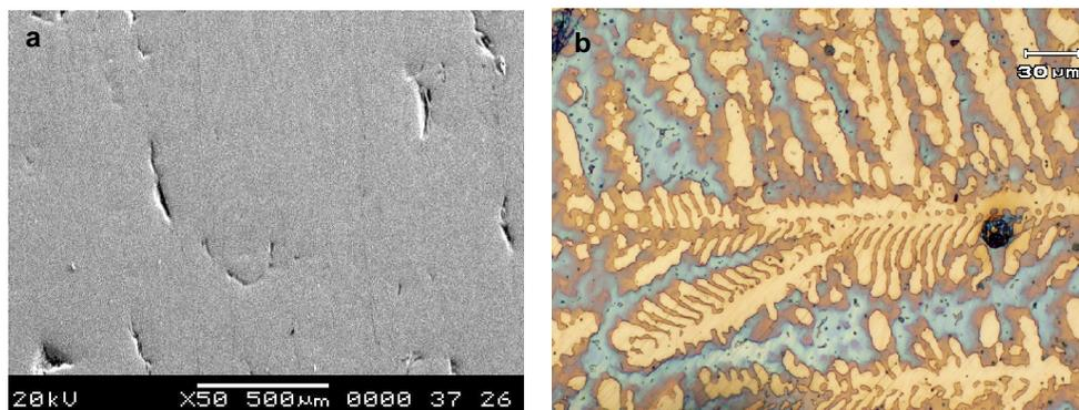
Figure 2. SEM and optical micrographs of as cast samples of Samarium-Cobalt ( $\text{SmCo}_5$ ). After polishing and etching shows (a) single phase microstructure (b) typical dendritic structure.
