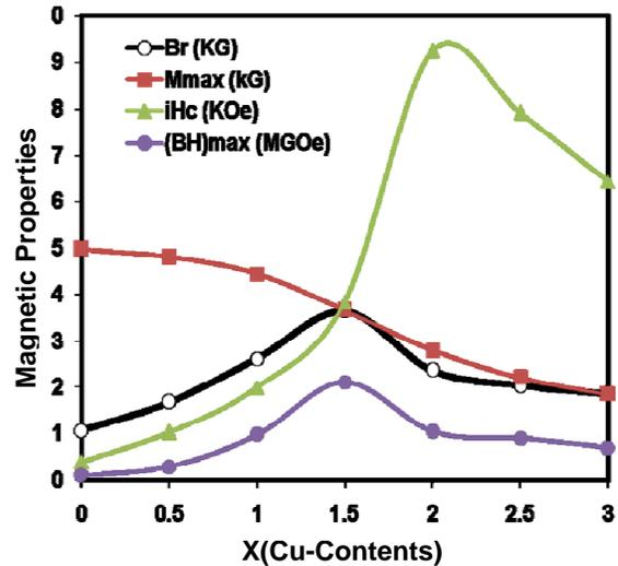
Figure 4. Magnetic properties of SmCo<sub>5-x</sub>Cu<sub>x</sub> as a function of copper contents.
