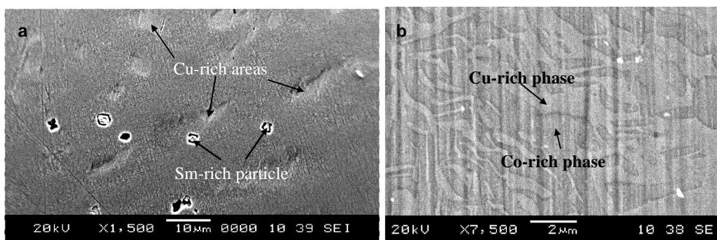
Figure 3. SEM micrographs of the sample  $\text{SmCo}_{1.5}\text{Cu}$ , with  $x = 1.5$  after polishing and etching. Samples reveal two-phase structures (a) as-cast (b) annealed at  $800^\circ\text{C}$  for 3hrs.
