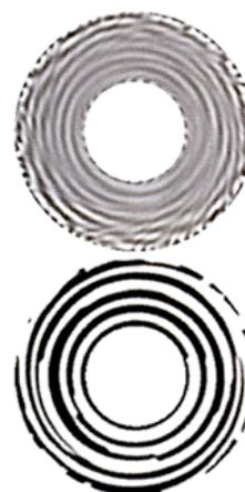
Figure 17. Simulation of a two-phase extrusion showing alternating concentric regions of each phase. Shown is the morphology after 1 s (top) and 20 s (bottom).
