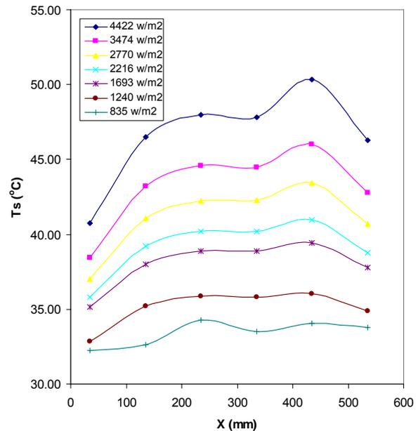
Figure 2. Surface temperature distribution along axial distance at different uniform heat fluxes.
