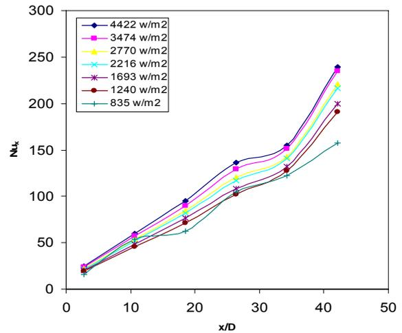
Figure 4. Local Nusselt number along dimensionless length  $x/D$  at different uniform heat fluxes.
