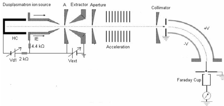
Figure 1. Schematic of experimental setup to analyze the energy of ion beam
