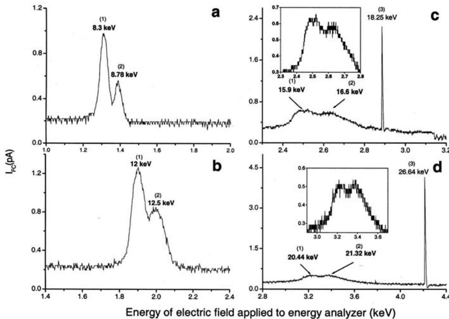
Figure 2. Energy spectra of ion beams at different energies (a) 12 keV (b) 17 keV (c) 22 keV (d) 27 keV.
