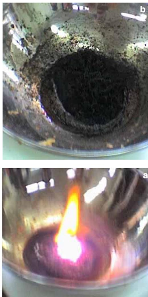
Figure 1 (a-b). Gel-combustion process for strontium iron cobalt based ( $\text{SrFe}_{0.5}\text{Co}_{0.5}\text{O}_3$ ) perovskite oxide powder. (a) Combustion at  $250^\circ\text{C}$  (b) Black brown powder collected after combustion.
