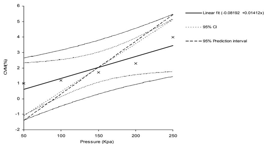
Figure 1. Manufacturer's coefficient of variation of pressure-compensating emitters with respect to different operating pressure of water source.
