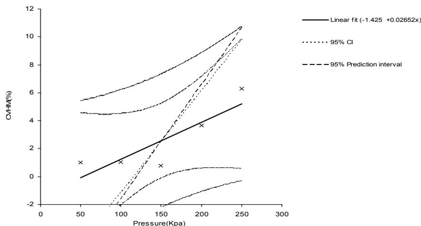
Figure 5. Total coefficient of variation of pressure-compensating emitters with respect to different operating pressure of water source.
