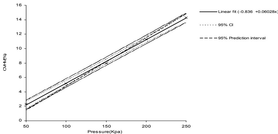
Figure 6. Total coefficient of variation of pressure-compensating emitters with respect to different operating pressure of water source.
