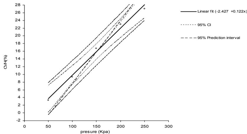
Figure 4. Hydraulic design's coefficient of variation of non pressure-compensating emitters with respect to different operating pressure of water source.
