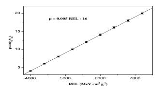
Figure 4. Calibration curve of reduced etch rate p vs *REL*. The points are the experimental data and the line is the best fit to the data point. The fitted equation is only valid in the *REL* range ~ 4000-7100 MeV cm<sup>2</sup>/g. The main contribution to the errors comes from the uncertainty in the determination of  $v_B$ . The uncertainties in the bulk velocity yield a systematic error on the reduced etch rate p.
