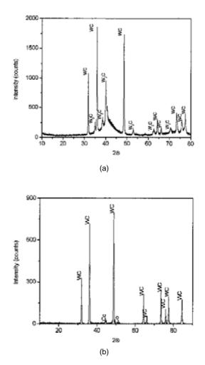
Figure 4. XRD analysis taken from HVOF sprayed coatings: Microstructured WC-10Co-4Cr coating; (b) Nanostructured WC-17Co coating.
