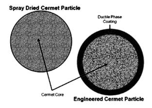
Figure 2. Schemiatic showing a comparison between the conventional spray dried powder particle and the novel "engineered" duplex Co-coated powder.
