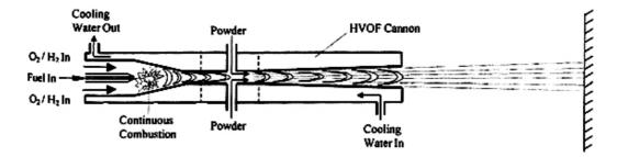
Figure 1. Schematic showing the HVOF spray gun.
