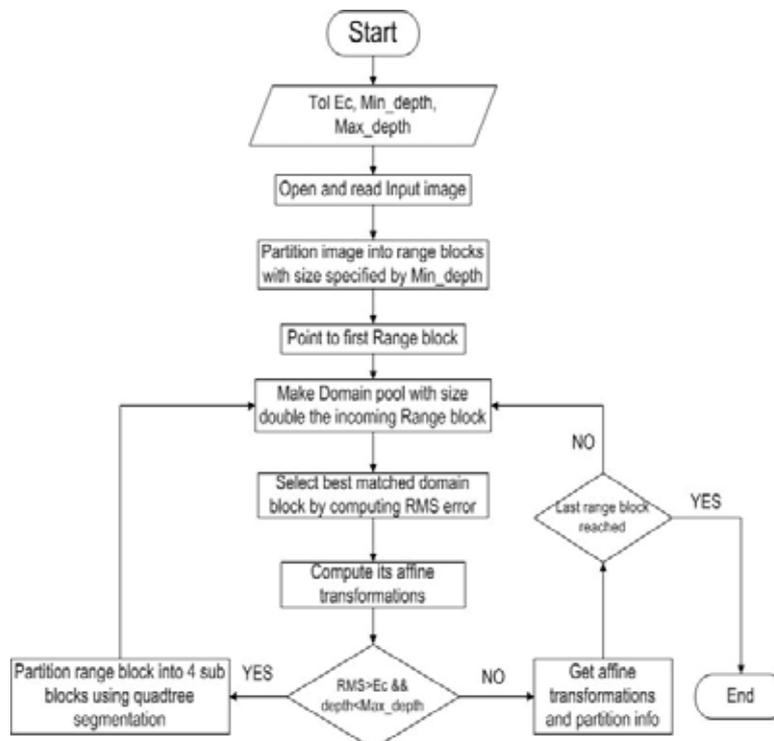
Figure 5. Flowchart for decoding process.
