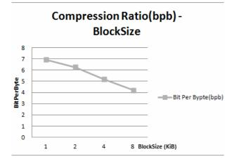
Figure 12. Block size affecting compression ratio measure in bits per byte.
