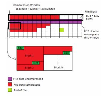
Figure 11. Accessing the unique file block after compression has been done on the file data.
