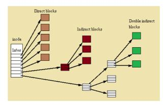
Figure 4. Block pointer addressing.
