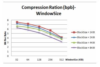
Figure 14. Compression ratio for different block sizes plotted against different window size selected for compression.
