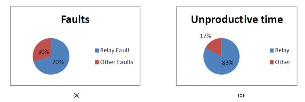
Figure 4. (a) Percentage of relay fault and other faults, (b) Percentage of unproductive time due to relays fault and other faults.
