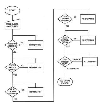
Figure 5a. Flow chart of the oil pumps start.
