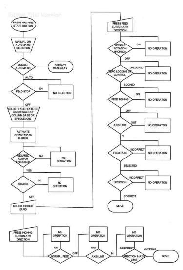
Figure 5c. Flow chart of the axis movement.
