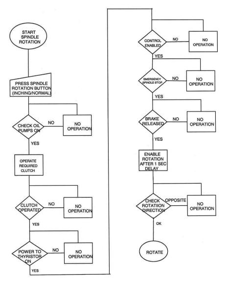
Figure 5b. Flow chart of the spindle rotation.
