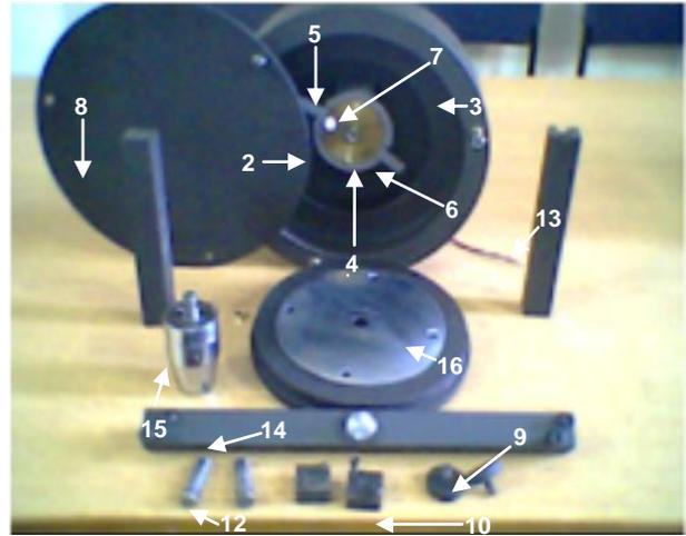
Figure 3. Detail of mechanical parts of test fixture.
