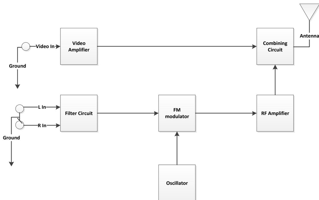
Figure 2. UHF / VHF TV transmitter block diagram.
