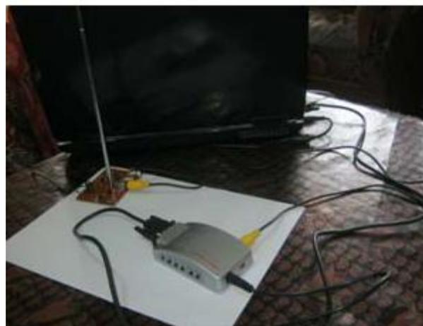
Figure 7b. VGA Converter.
