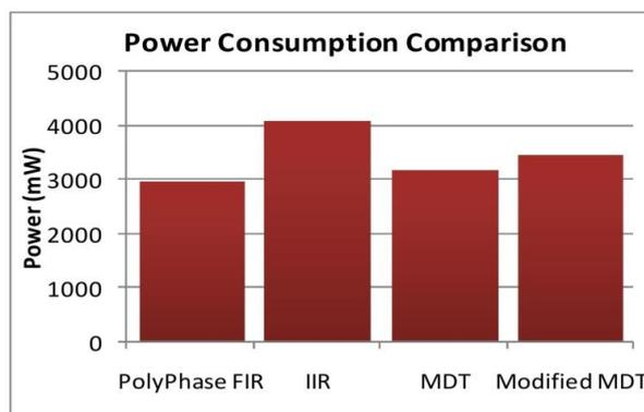
Figure 12. Power consumption of four architectures in mW.
