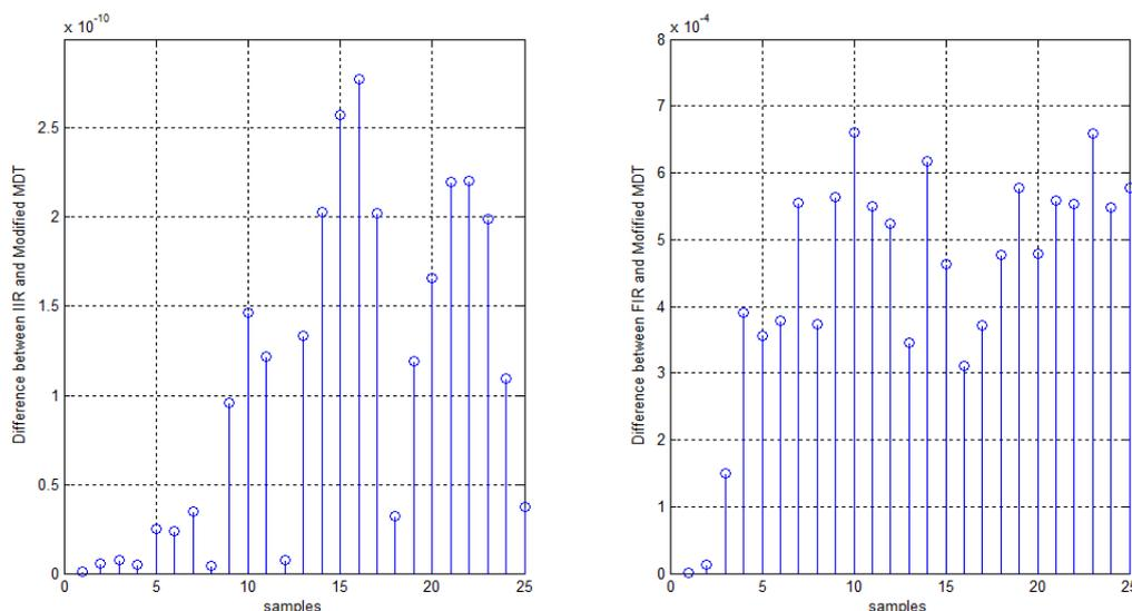
Figure 10. The difference between outputs of IIR vs. modified MDT and FIR vs. modified MDT filters.
