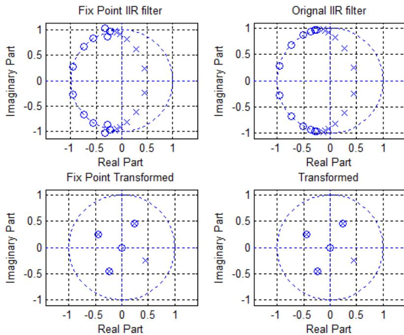
Figure 13. Pole zero plot of IIR Decimation filter and Modified MDT Decimation filter.
