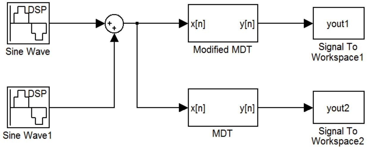
Figure 6. Modified MDT and MDT decimation filter comparison architecture.
