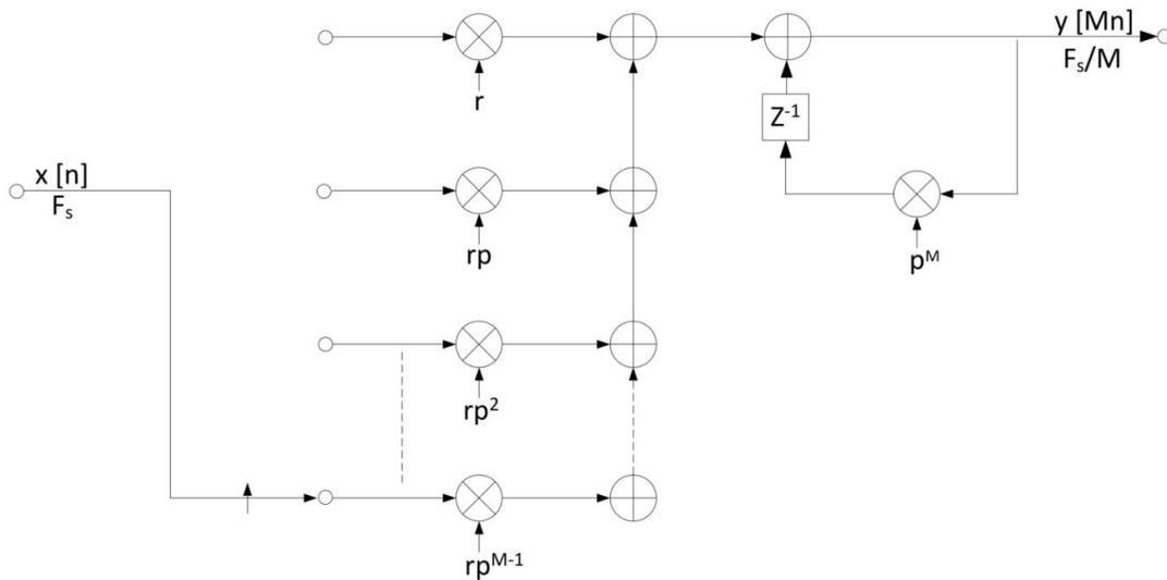
Figure 1. Decimator filter obtained by MDT on first order recursive filter [5].
