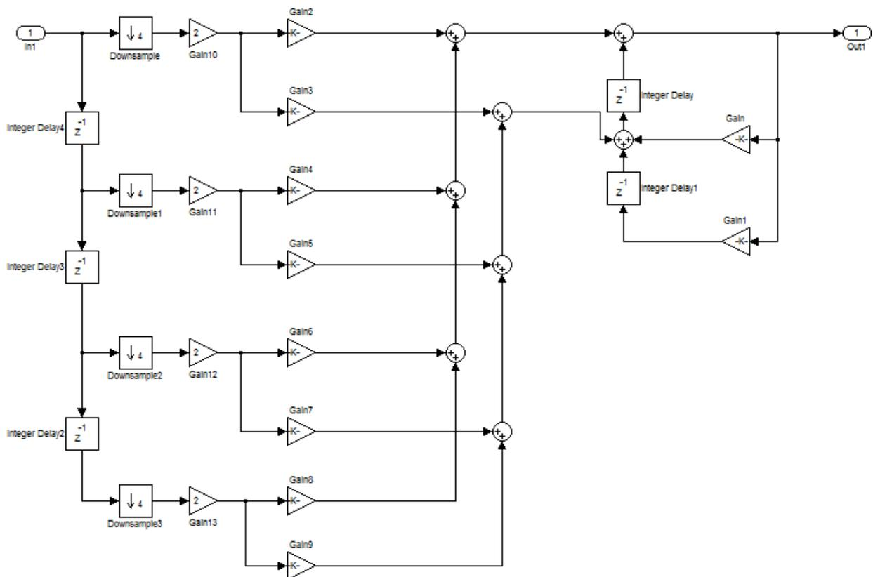
Figure 7. MDT decimation filter internal structure.
