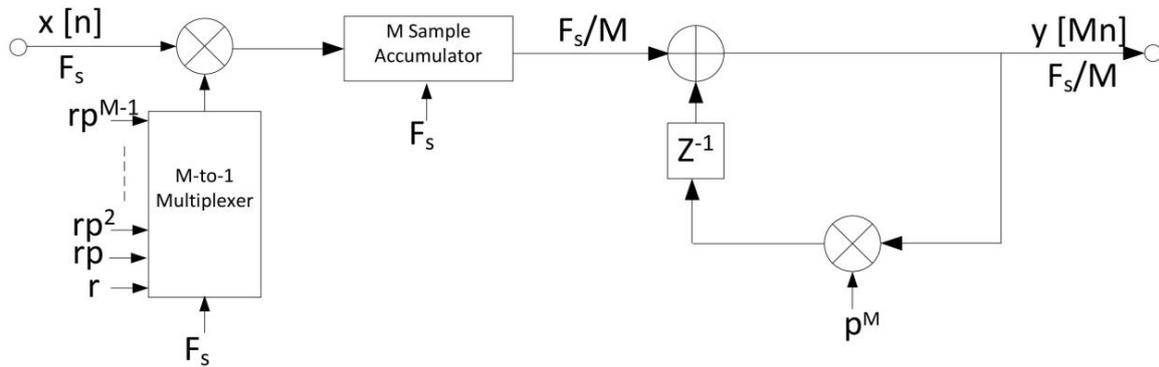
Figure 4. Modified MDT Decimation filter obtained from first order recursive filter.
