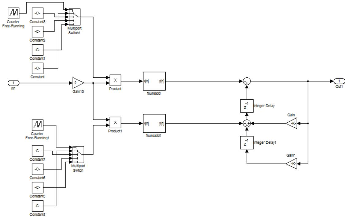
Figure 8. Modified MDT decimation filter internal structure.
