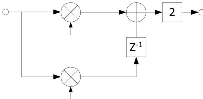
Figure 3. Sub filter  $H_k(z)$  Unfolded with coefficients from [4].
