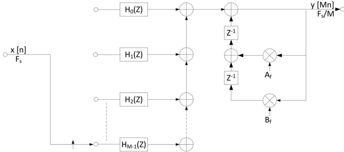
Figure 2. Decimator filter obtained by MDT on second order recursive filter [5].
