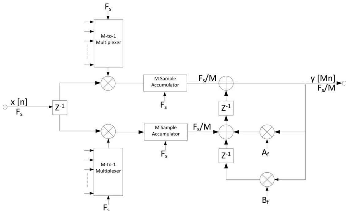
Figure 5. Modified MDT decimation filter obtained from second order recursive filter.
