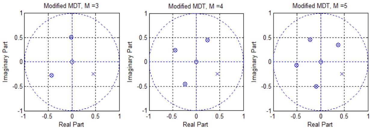
Figure 16. Pole zero plot for Modified MDT Filter for varying M.
