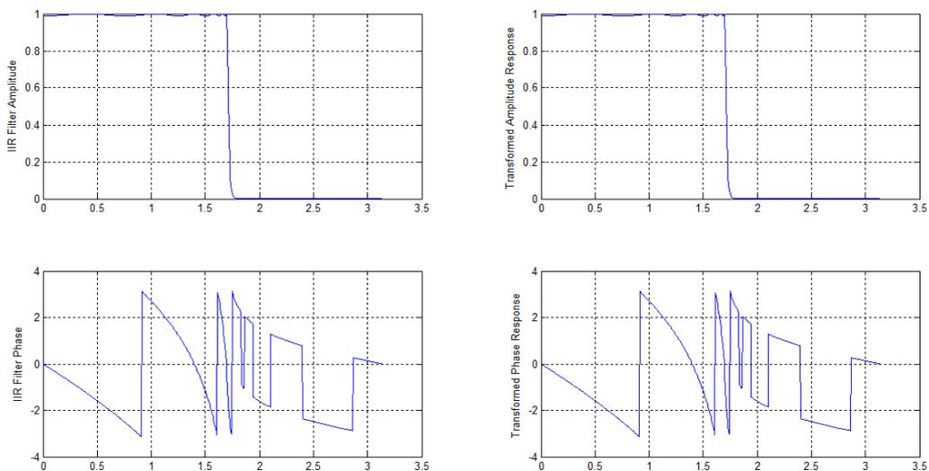
Figure 14. Magnitude and Phase responses of IIR and Modified MDT Decimation filters.
