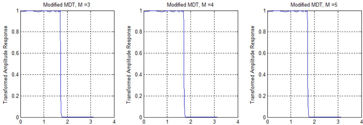
Figure 15. Amplitude Response of Modified MDT Filter for varying M
