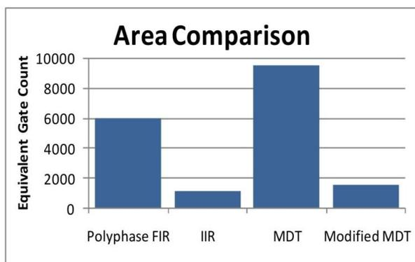
Figure 11. Hardware area comparison of different architectures in terms of equivalent gate count.
