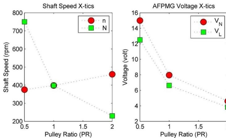
Figure 12. WES model results on variable PR
