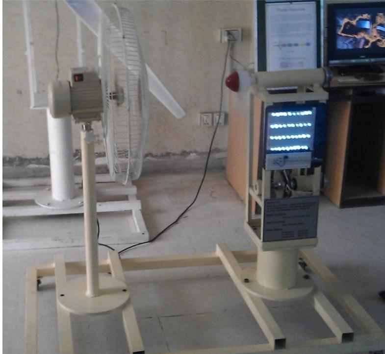
Figure 9. Operational micro WES model in lab.
