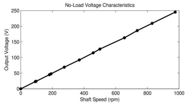
Figure 8. No-load test.
