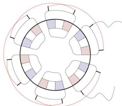
Figure 4. Coil-magnet overlapping for begin-to-end connection.
