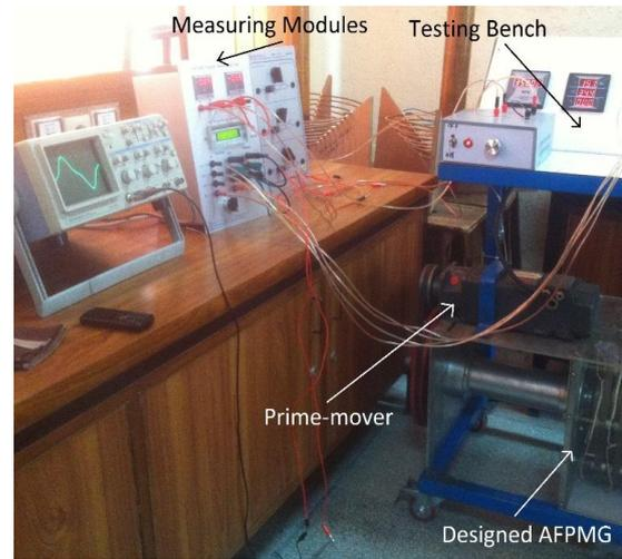
Figure 7. Generator testing bench.
