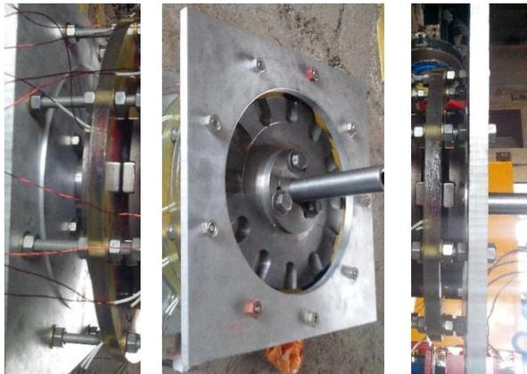
Figure 6. Complete AFPMG assembly and model.
