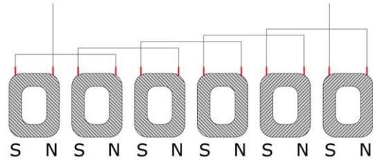
Figure 2. Begin-to-end winding pattern.
