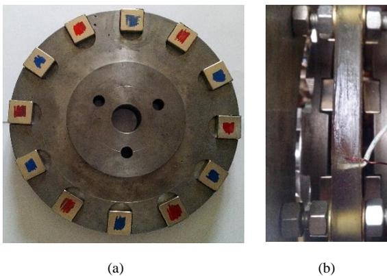
Figure 5. (a) Rotor disc, (b) Stator disc sandwiched between rotor discs.
