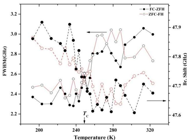
Fig. 4. Temperature dependent Brillouin spectra parameters measured under: (i) zero-field heating (ZFH) condition after field cooling (FC), (ii) field heating (FH) after zero-field cooling (ZFC) of the specimen.
