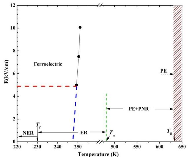
Fig. 1. Temperature-electric field phase diagram of PLZT- $x/65/35$  ceramics [5], abbreviations used are explained in the text.
