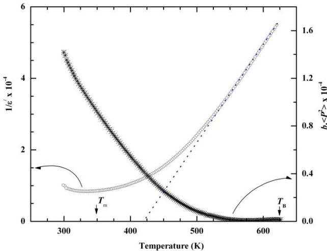
Fig. 2. Plot of inverse dielectric constant ( $\epsilon'$ ) and calculated local polarization compounded with dielectric nonlinearity coefficient ( $b$ ) as a function of temperature for PLZT-10/65/35 ceramic.
