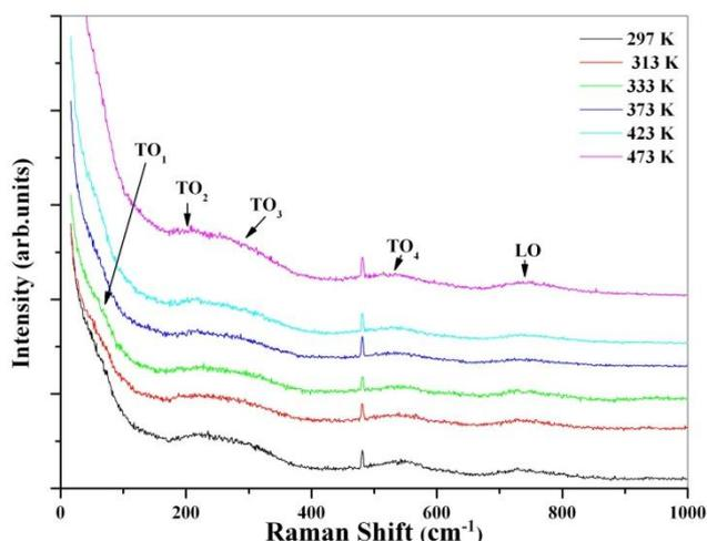
Fig. 3. Raman spectra of PLZT-10/65/35 ceramic specimen measured at some selected temperatures. Presence of different optical phonon modes is indicated by arrows.
