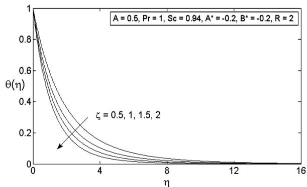
Fig. 5. Temperature profiles for different  $\zeta$  .
