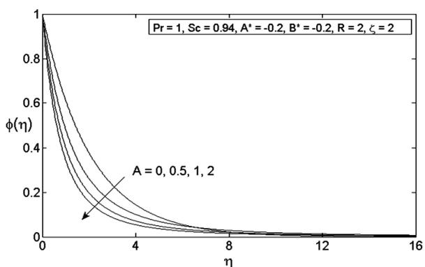
Fig. 3. Concentration profiles for different  $A$  .
