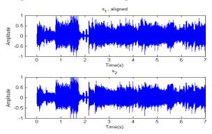
Fig. 8: Sample-to-sample aligned signals after cross-correlation
