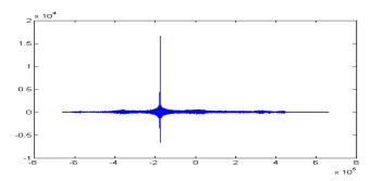
Fig. 7: Correlation between signals (finding lead/lag time of signal w.r.t reference signal)
