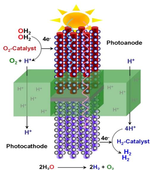
Fig. 7: A conceptual design of the artificial leaf proposed by JCAP based on arrays of light harvesting nano-/micro-wires, embedded in a proton-conducting membrane, coated with O<sub>2</sub> and H<sub>2</sub> evolving catalysts from water splitting reaction
