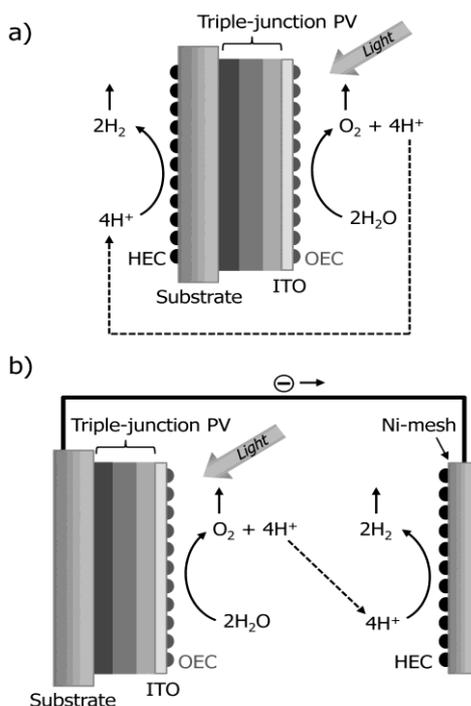
Fig. 6: (a) A working model of an artificial leaf with a triple-junction amorphous/microcrystalline Si system as reported by Miller and Nocera; (b) A wired-configuration for the PEC based water oxidation system
