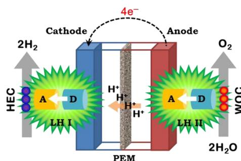
Fig. 1: Schematic presentation of a solar-fuel device showing light-harvesting (LH), water oxidation (WOC) and H<sub>2</sub> evolution catalyst (HEC). The anode and cathode are separated by proton exchange membrane (PEM). (A and D represent donor-acceptor pair)
