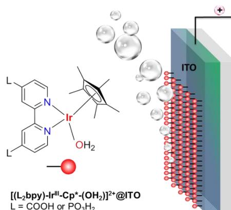
Fig. 5: A surface immobilized electrochemical water oxidation assembly showing Cp\*-Iridium derived complexes with  $\text{L}_2\text{bpy}$  ( $\text{L}=\text{COOH}$ ,  $\text{PO}_3\text{H}_2$ ) ligands for electro-driven oxygen evolution
