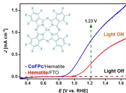
Fig. 3: Linear sweep voltammograms under dark (dashed lines) and full light illumination (solid lines) for hematite (red lines) and hematite/CoFPc (blue lines) systems in 0.1 M NaOH (pH=13; scan rate  $10 \text{ mV s}^{-1}$ )
