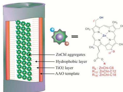
Fig. 2: Schematic view of alkyl-TiO<sub>2</sub>-coated AAO nanochannel templates (AAO-Ti-C<sub>13</sub>) and imprinting of self-assembled zinc chlorophyll aggregates (AAO-Ti-C<sub>13</sub>ZnChl)
