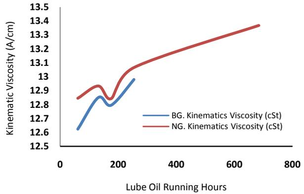
(b) Variation in kinematic viscosity with lube oil running hours
