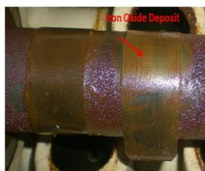
(c) Deposition of FeO on Cam Shaft
