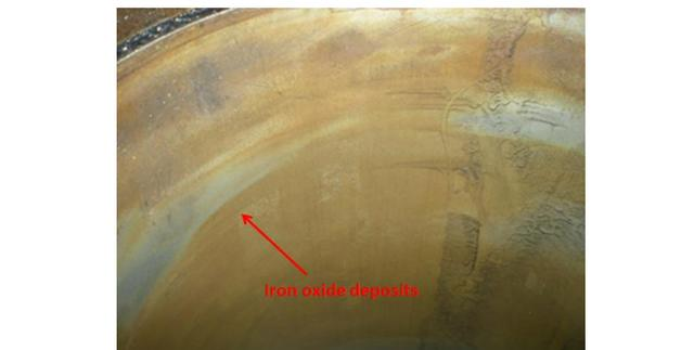
Fig. 4: The iron oxide deposits on the internal surface of the cylinder liner with natural gas as fuel
