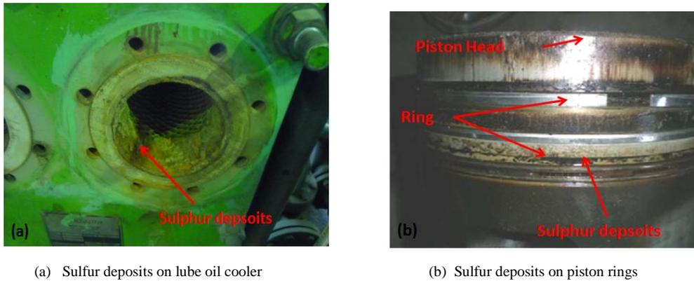
Fig. 3: Sulfur deposits in lube oil circuit with biogas as a fuel
