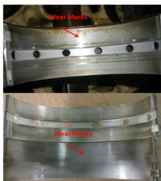
(a) Worn out Shell Bearing
