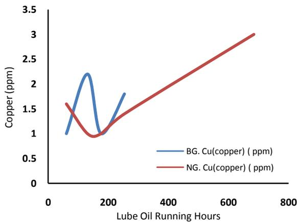
(e) Variation in Cu debris with lube oil running hours
