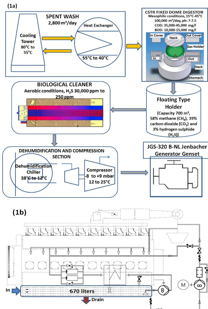
Fig. 1: (a) Schematic diagram of biogas generation starting with mixing of spent wash with cow dung, followed by anaerobic digestion, then by bacteria assisted biological purification, followed by chilling compression in heat exchangers and loading into the JGS-320 B-NL Jenbacher, (b) Lube oil circulation circuit diagram for JGS-320 B-NL Jenbacher generator Genset which was employed in the experimental study
