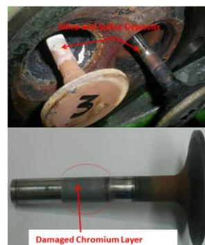
(b) Deposition and Damage of Valves and Seat Area
