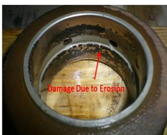
(e) Eroded Connecting Rod
