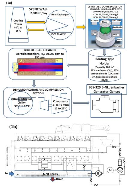
Fig. 1: (a) Schematic diagram of biogas generation starting with mixing of spent wash with cow dung, followed by anaerobic digestion, then by bacteria assisted biological purification, followed by chilling compression in heat exchangers and loading into the JGS-320 B-NL Jenbacher, (b) Lube oil circulation circuit diagram for JGS-320 B-NL Jenbacher generator Genset which was employed in the experimental study
