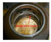
(e) Eroded Connecting Rod
