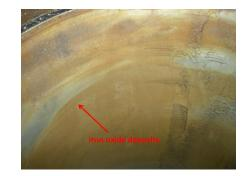
Fig. 4: The iron oxide deposits on the internal surface of the cylinder liner with natural gas as fuel
