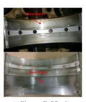
(a) Worn out Shell Bearing
