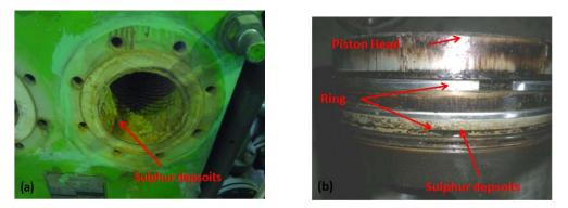
(a) Sulfur deposits on lube oil cooler
