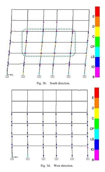
lateral load of 1250 kips and lateral displacement of 2.81 ft. The performance point of the building lies between life safety and the collapse prevention, indicating considerable seismic damage potential in the building requiring appropriate seismic retrofitting.
