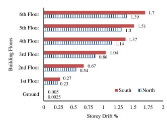
Fig. 6: Lateral storey drift ratios.
