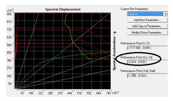
Fig. 5: Capacity spectrum of model building.
