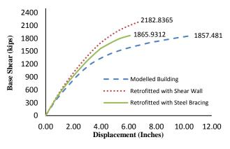
Fig. 11 Capacity Curves for 2.5% drift of Model Building and Retrofitted Building.
