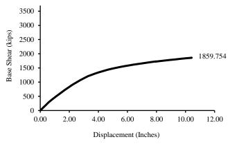
Fig. 4: Capacity curve for 2.5% drift of model building.
