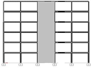
Fig. 7: Retrofitted with shear wall.
