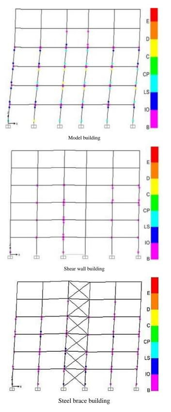
Fig. 10: Plastic hinge formation in south grid of Zone 3.
