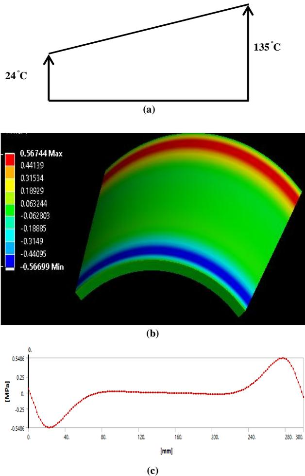
Fig. 1: (a) linear temperature in axial direction. (b) and (c) thermal stresses (MPa) generate in tube due to linear temperature distribution.
