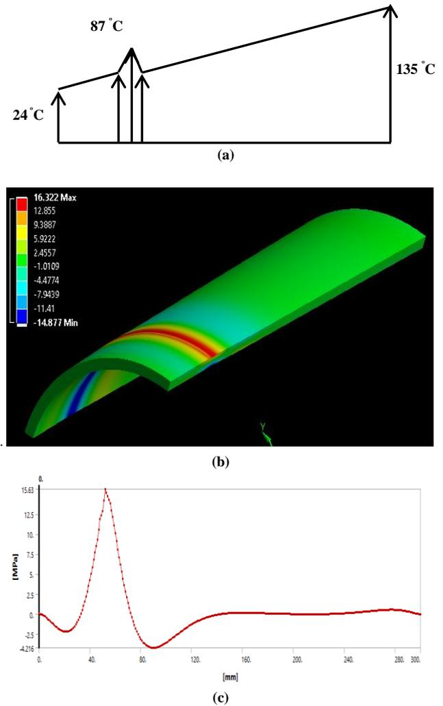
Fig. 2: (a) Nonlinear temperature distribution, (b) and (c) show thermal stresses (MPa) produce due to nonlinear temperature in axial direction of tube.
