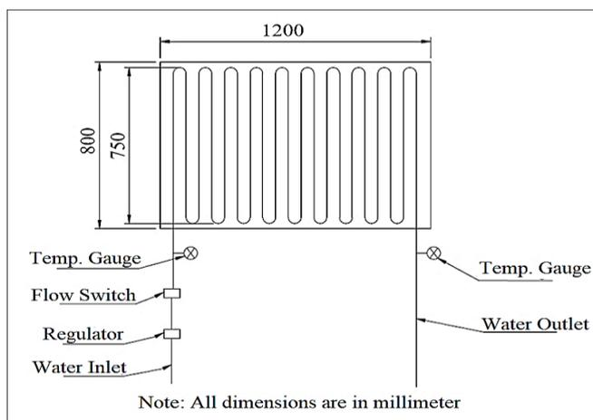
Fig. 2: Schematic of heat recovery system.
