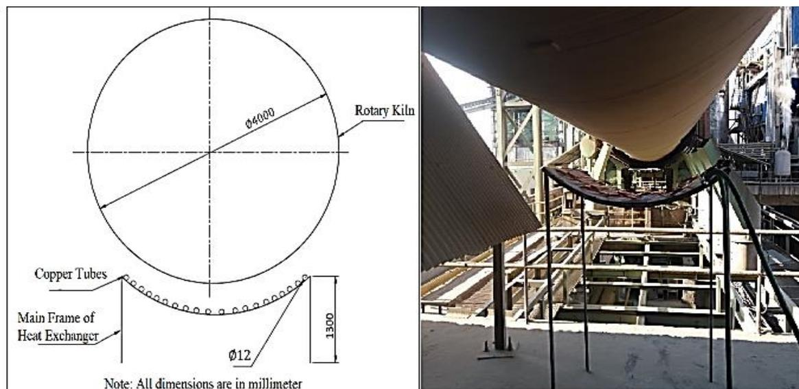
Fig. 4: Schematic and actual views of experimental setup.
