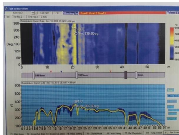
Fig. 3: Kiln scanner view showing temperature variations.
