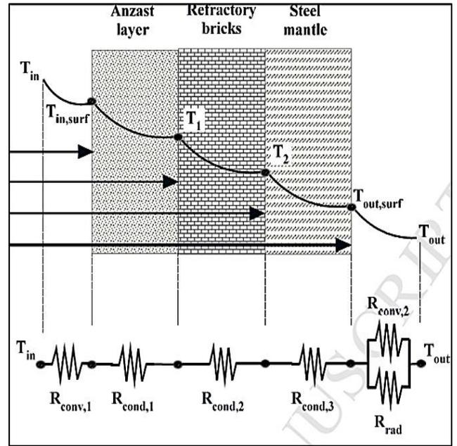
Fig. 1: Modes of heat transfer at rotary kiln [4].
