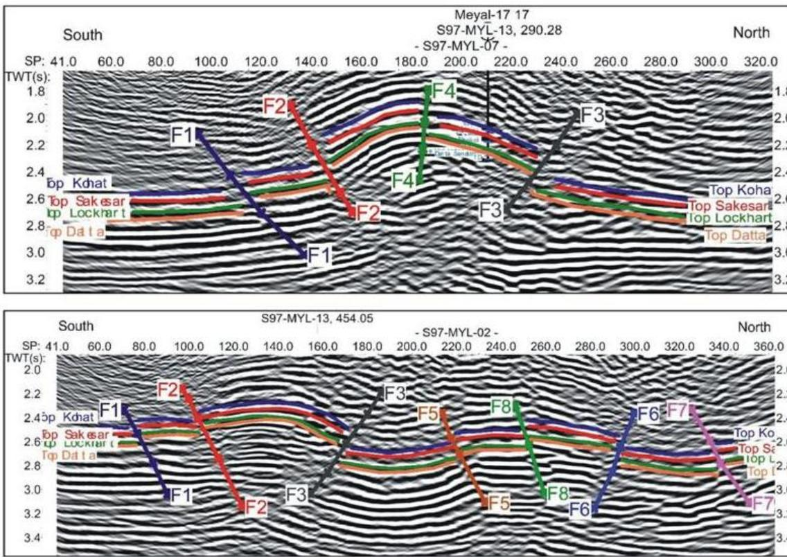
Fig. 4: Marked horizons and faults on N-S dip oriented seismic line S97-MYL-07 (upper) and S97-MYL-02 (Lower)
