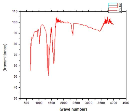
Fig.1: FT-IR spectrum of synthesized silver nanoparticles by using leaves extract of *S. cumini*
