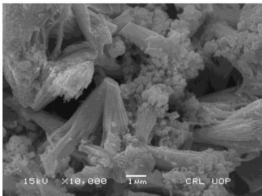
Fig.3: SEM analysis of synthesized silver nanoparticles by using leaves extract of *S. cumini*
