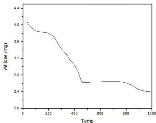
Fig. 4: TGA analysis of synthesized silver nanoparticles by using leaves extract of *S. cumini*
