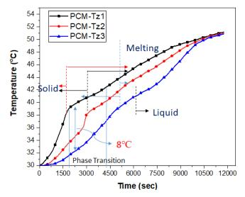
Fig. 5: Temperature profile of pure paraffin along z-axis
