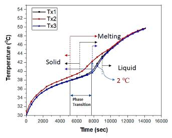
Fig. 8: Temperature profile of Iron-Nickel foam/paraffin composite along X-axis.
