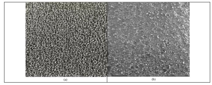
Fig. 3: Images of (a) Pure iron-nickel foam and (b) Iron-nickel foam PCM composite.
