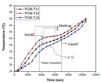
Fig. 4: Temperature profile of pure paraffin along x-axis
