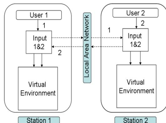
Fig. 3. Architecture/Framework of collaborative virtual environment
