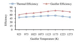
Fig. 7: Gasifier and thermal efficiency verses gasifier temperature
