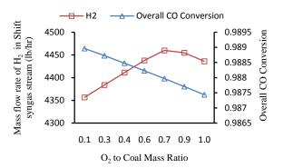
Fig. 4:  $H_2$  mass flow rate and CO conversion verses  $O_2$  to coal mass ratio.
