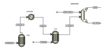
Fig. 3: Aspen Plus flow sheet model for production of H<sub>2</sub>-enriched syngas from gasifier exhaust gas stream
