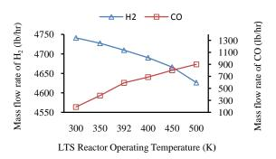
Fig. 5: Mass flow rate verses LTS reactor operating temperature
