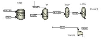
Fig. 2: Aspen Plus flow sheet model for fixed bed gasifier
