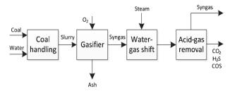
Fig.1: Simplified block flow diagram for hydrogen production
