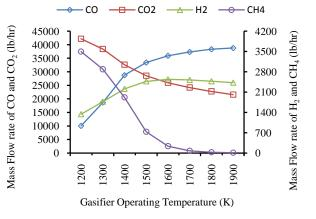
Fig. 6: Mass flow rate verses gasifier operating temperature
